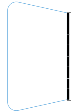
One-way horizontal air discharge to the left
